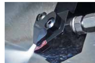
Coolant through spindle system
