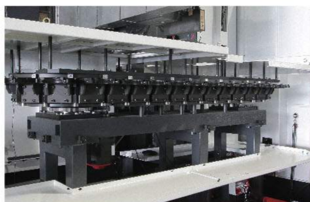
Tool magazine for 32, 48, 60 tool position
