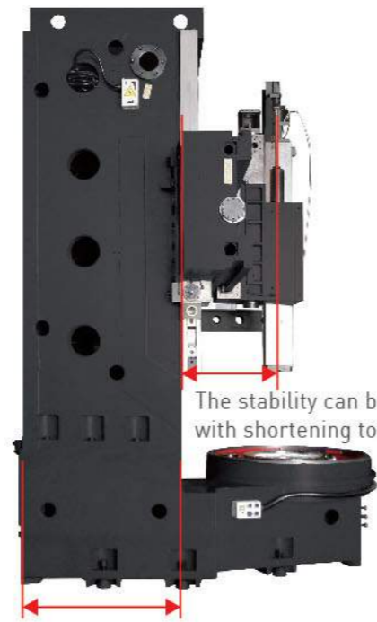
Thickness increased to guarantee structural rigidity.
