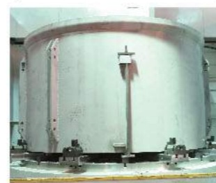
VTL3000ATC+ C Wind power generator-stator machining
