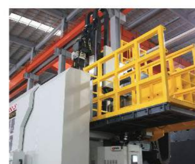
Operator's platform extension
