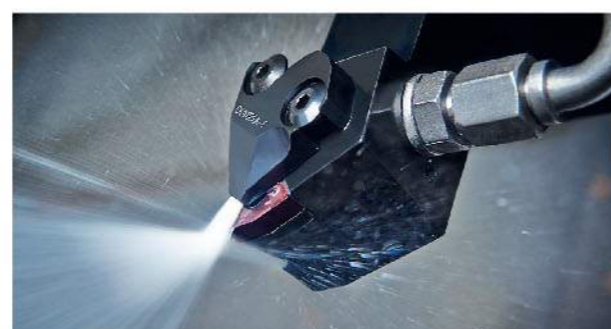
Coolant through tooling 12/20/60/ bar
